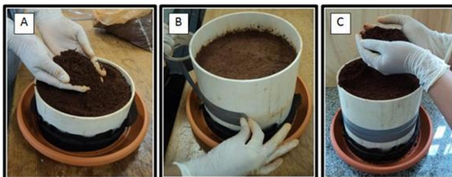
Figure 5. Implementation of the experimental unit: Filling the lower cylinder with soil at the density of 1.0 Mg m -3 (A); Joining both cylinders with duct tape, showing the compacted layer (B); Filling the remaining volume of the upper cylinder above the compacted layer at the density of 1.0 Mg m -3 (C).
